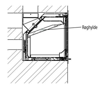
The smoke turn plate is removed by lifting at one side after which it will come clear of the other side and be taken down into the combustion chamber and out through the door. Similarly, it is put in place by moving it up askew at one side and then at the other side, and it is then put in place in the middle.
