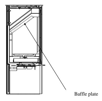
Each smoke baffle plate is to be removed separately. Both smoke baffle plates are removed by lifting up at one side after which they may come clear at the other side and be taken down into the combustion chamber and out of the door. Similarly, they are put in place by leading them up slanting-wise at one side, and then at the other side, and they are then put into place in the middle.
