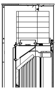
Each smoke baffle plate is to be removed separately. Both smoke baffle plates are removed by lifting up at one side after which they may come clear at the other side and be taken down into the combustion chamber and out of the door. Similarly, they are put in place by leading them up slanting-wise at one side, and then at the other side, and they are then put into place in the middle.
